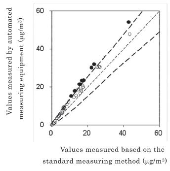
Figure 1 Image of equivalent test for automatic monitor Bold broken lines show control limit area. Open and closed circles show data within and out of acceptable range, respectively.
